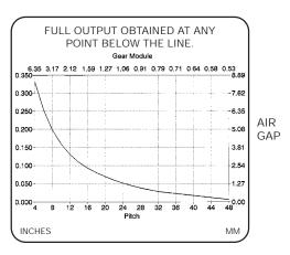
FOR APPLICATIONS REQUIRING VERY LOW SPEED RESPONSE AND/OR SENSING OF FINE PITCH GEARS. ALL SENSORS HAVE SEALED SENSING AREA. ALIGNMENT NOT REQUIRED. 300 SERIES SSTL HOUSING.
